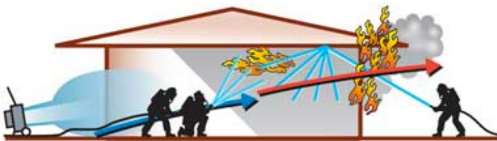
Figure 9. Transitional, Positive-Pressure Attack, and Gas Cooling
