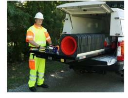
still in service, and they are transferable from one unit to another. One person can easily operate it when needed, and its use keeps the operator safer as he or she can remain on the side of the truck away from oncoming vehicles. Its use has also reduced on the job injuries as equipment is accessible without having to execute awkward lifts from the truck bed or climb in and out of the bed.
